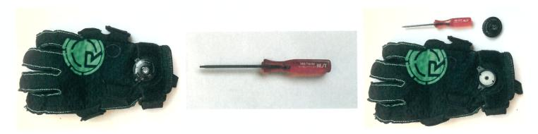
Unscrew the Boa reel cap using a T-6 Torx Screwdriver. The screw is located in the center of the face of the Boa cap in the letter O of Boa
