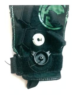
Extract the Boa inner spool by lifting it straight up. Then feed the Line through the ratchet lace opening
