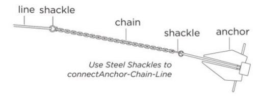
Chain keeps anchor in correct setting postion for a stronger hold
